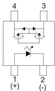
**Wiring Diagram 接线图**
