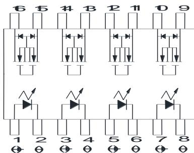
**Wiring Diagram 接线图**
